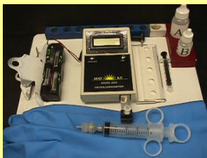
Figure 2. New Horizons PROFILE luminometer and necessary equipment.
