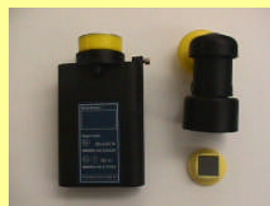
Figure 3. Novel Personal air sampler CIP-10M
