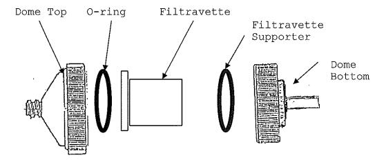
The dome top has a luer-lok to which a syringe can be affixed and the contents of the syringe filtered through the Filtravette. The black 0-ring must be in place or it will leak. It's advisable to use a syringe protective tip on the Dome Bottom tip of the Cell Concentrator when not in use.
