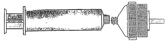
Push the Sample Through the Cell Concentrator by Applying Moderate Pressure to the Syringe Plunger, Concentrating the Cells on the Filtravette<sup>TM</sup> Membrane
